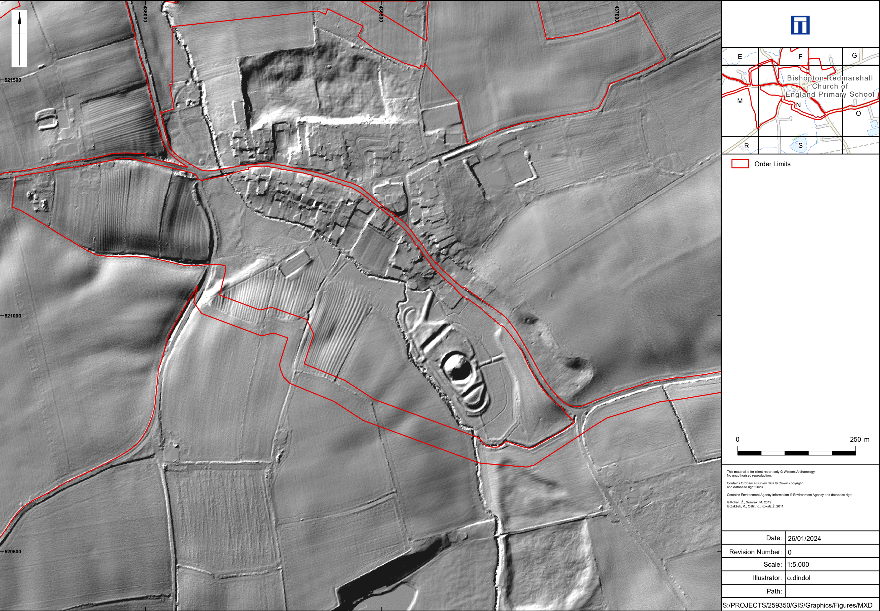
Site, location and Analytical hillshade (Illumination angle 315°) derived from input spatial resolution of 1m DTM (Sheet N)
