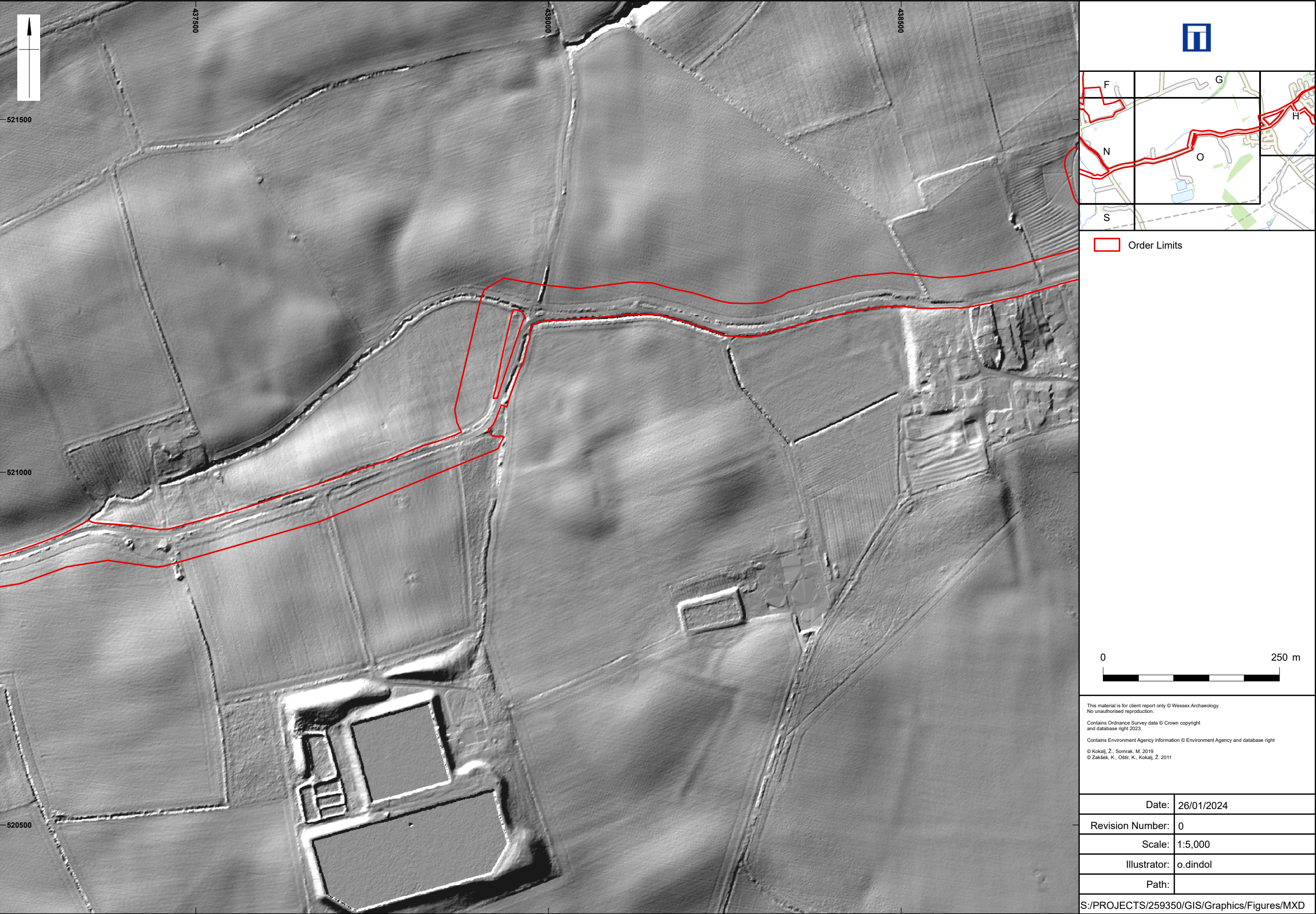
Site, location and Analytical hillshade (Illumination angle 315°) derived from input spatial resolution of 1m DTM (Sheet O)
